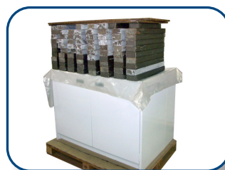
Actual photo during Cabinet Load Testing
