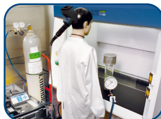
Tracer Gas (SF 6 ) Containment Test
