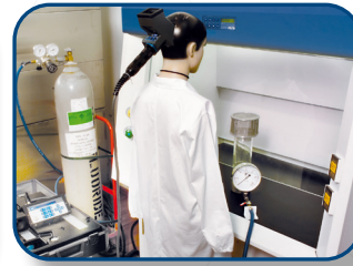
Tracer Gas (SF 6 ) Containment Test
