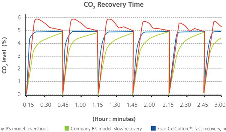
Figure 2. Precisely tuned sensor and software results in faster recovery of CO<sub>2</sub> without overshoot. This ensures uniform CO<sub>2</sub> levels even with frequent incubator door openings.
