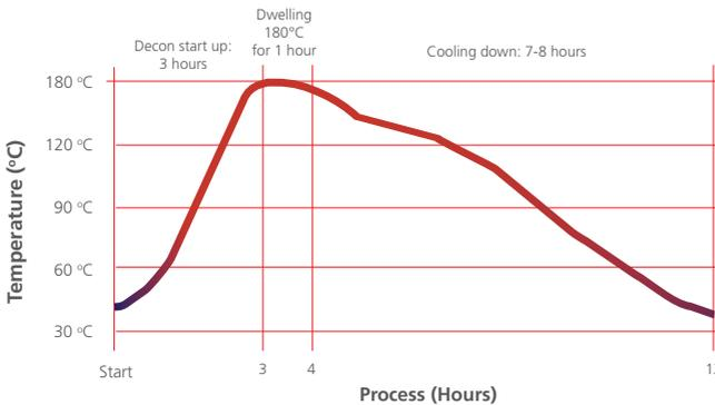
Figure 4. Graph of a full cycle sterilization process. Complete cycle lasts up to 12 hours.
