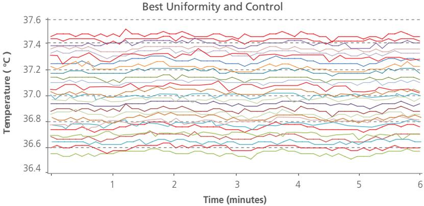
Figure 1. Different lines represent 27 sensors positioned inside the chamber. Esco CelCulture® CO<sub>2</sub> incubator has uniformity variance of less than  $\pm 0.5$  which means all the samples are evenly heated.\*
